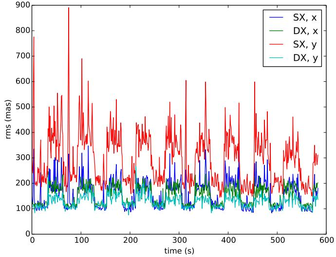
Figure 5: Jitter error with the vibration compensation turned on and off every 30 seconds
