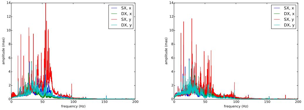
Figure 6: Vibration spectrum before (left) and after (right) the fast link improvement
