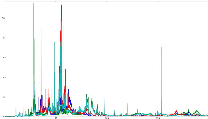
Figure 1: Vibration spectra of accelerometer on LM1 (SX side); averaged measurements, March 2017; x: frequency (Hz), y: accelerometer output
