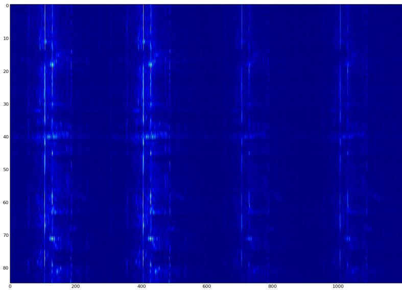
Figure 3: Frequency 28.5 Hz line for all 4 accelerometers on LM1 (SX); x: frequency cuts around the line for all four accelerometers; y: different data sets
