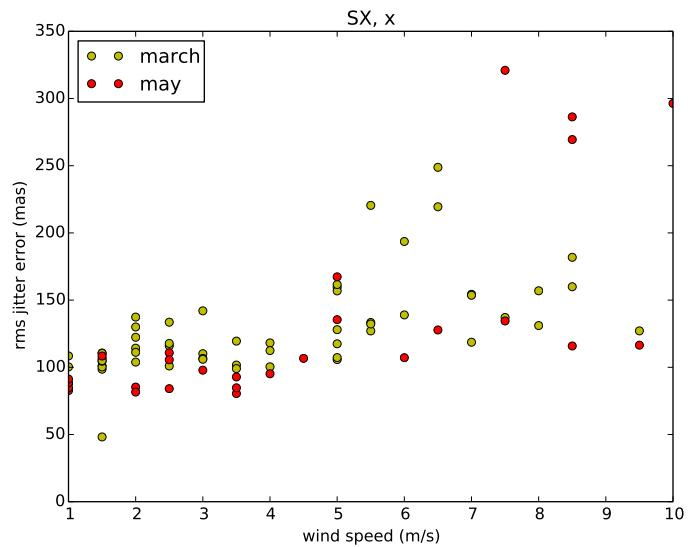
Figure 7: Jitter error before (march) and after (may) the fast link improvement vs. wind speed
