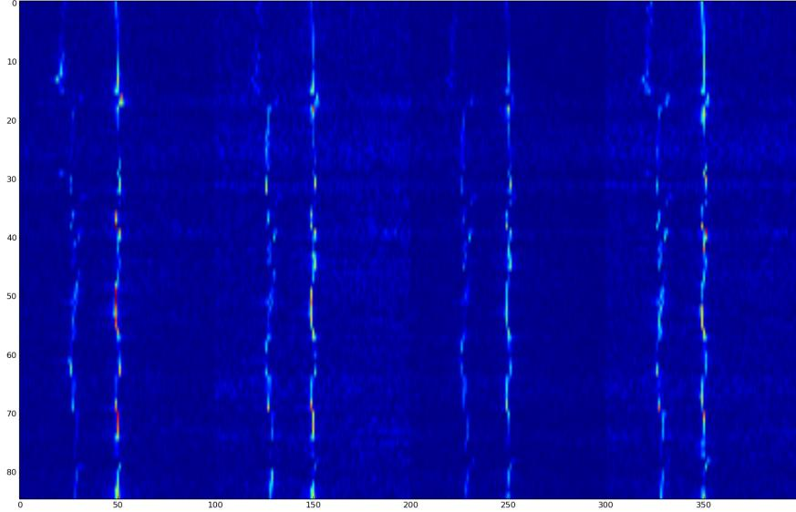
Figure 4: Frequency 97.5 Hz line for all 4 accelerometers on LM1 (SX); x: frequency cuts around the line for all four accelerometers; y: different data sets
