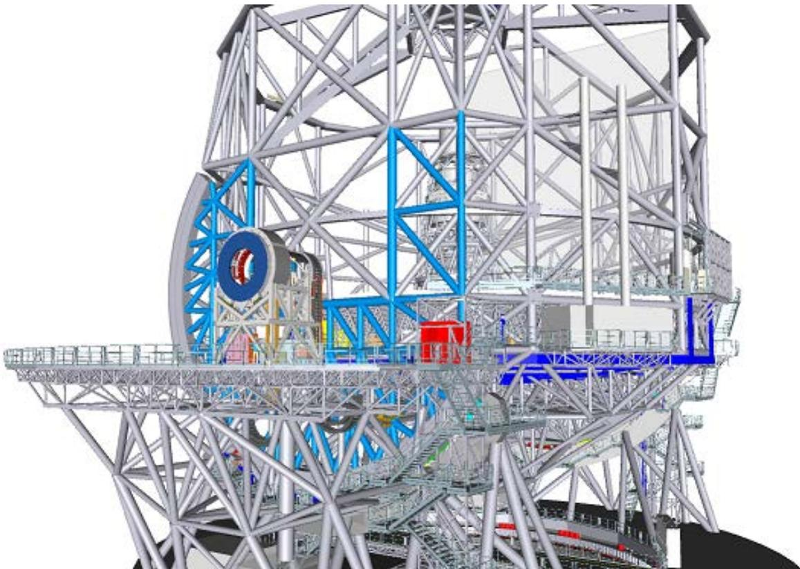
Figure 1: 3D sketch of the Prefocal Station on the ELT Nasmyth platform.
