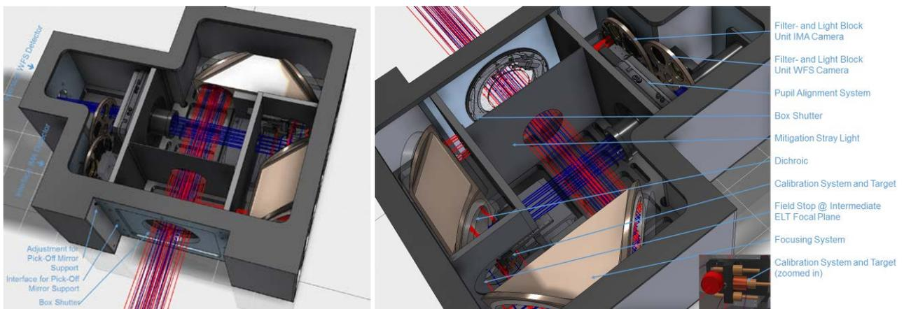
Figure 5: CAD model of the Optical Box of the SA: the trombone (Focusing System) keeps the focal plane of ELT in the same position inside the Optical Box (Intermediate ELT Focal Plane in the figure). A calibration unit system can be inserted on the intermediate ELT focal plane. The pupil reimaging lens is mounted on lateral translation stages, which allows to center the pupil on the detector (Pupil Alignment System).
