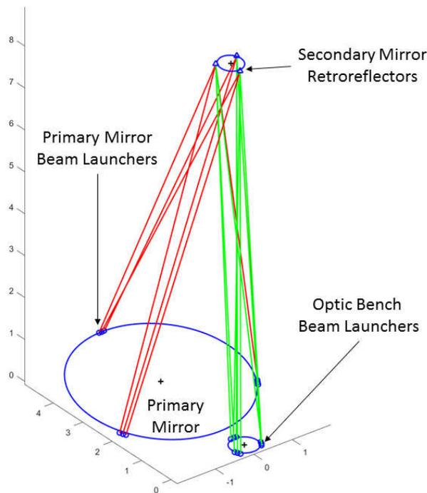
**Figure 3: HabEx laser metrology truss. Beam launchers are placed at the primary and tertiary mirrors and reflect from common retroreflectors located at the secondary mirror. The primary and secondary mirrors are mounted on rigid body actuators which are actively controlled in closed loop with laser metrology. Laser metrology truss**
