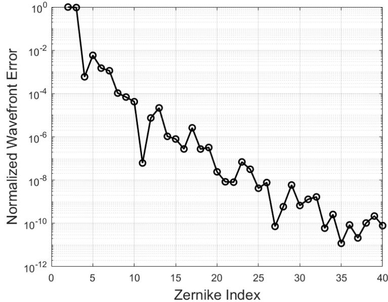
Figure 6: A charge 6 vector-vortex coronagraph is insensitive to low-order Zernike terms Z1-Z8 and Z11, but is not effective in suppressing the higher order terms. The worst offenders, Z2 and Z3, line-of-sight errors, are corrected by the fine guidance control loop. For the unobscured HabEx design, high order Zernike terms, due to rigid body motion of the primary and secondary mirrors, are not produced with amplitudes large enough to affect the contrast.
