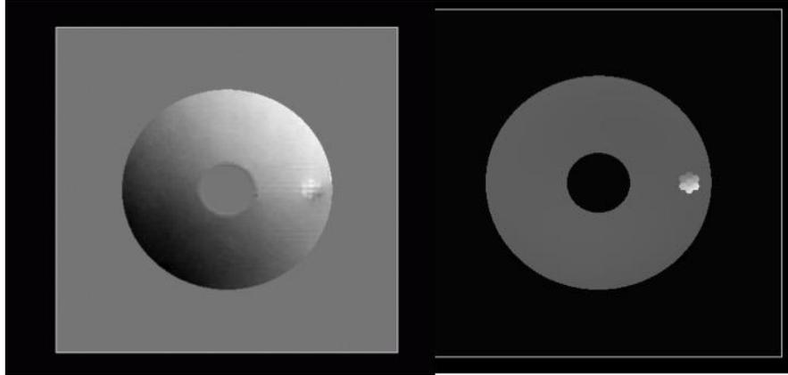
**Figure 1: On the left, difference between the DM shapes with and without the tilted segments. On the right, shape of the phase screen with tilted segments.**
