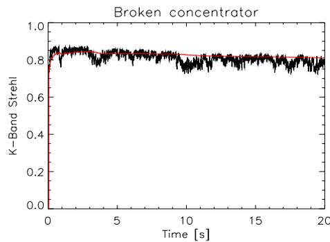
**Figure 2: Strehl as a function of time, when the concentrator breaks and slowly tilts towards its final position.**
