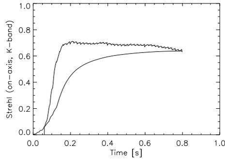
**Figure 5: Strehl as a function of time, for a PYR WFS correction with 0 pyramid modulation.**
