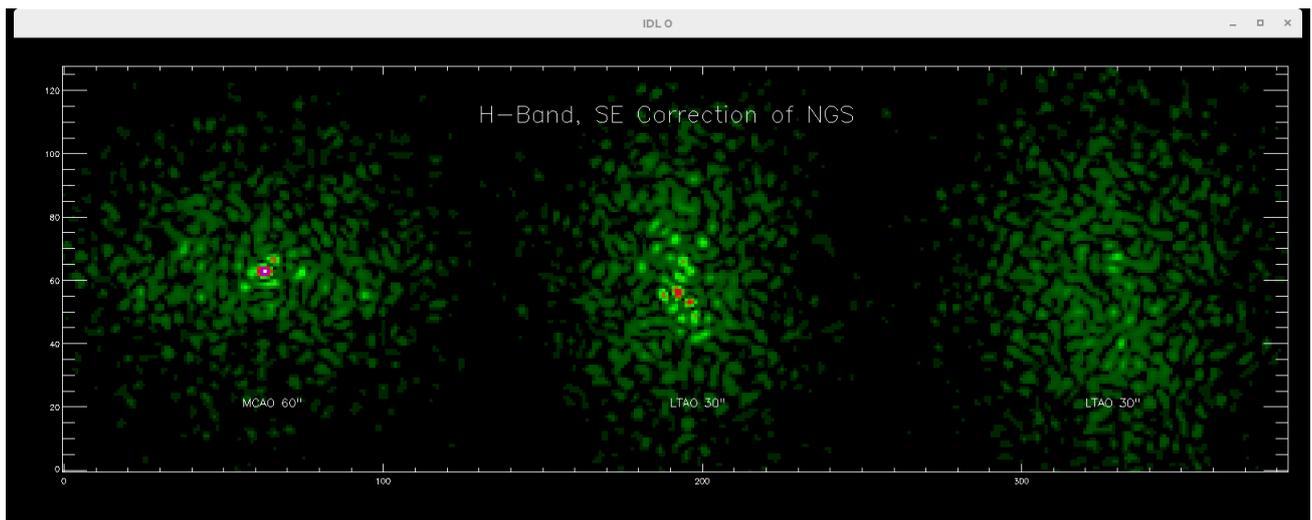
**Figure 6: Effect of correcting the TT star with AO: on the left, with MCAO (some degree of correction is observed off-axis), LTAO (30'' from the axis) and LTAO at 60'' off-axis, where correction by the AO (due to central optimization) is small.**
