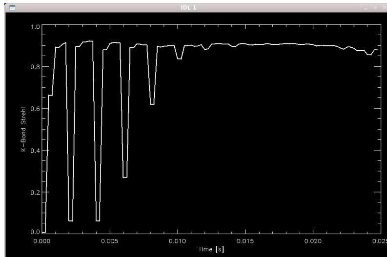
Figure 3: Strehl ratio (K-band) as a function of time, for the cascaded AO system.
