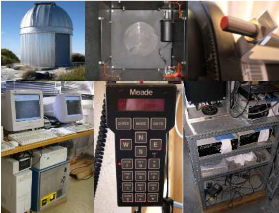
FIGURE 2.3— Different views of the STARE instrument. From top left to bottom right: dome, telescope shutter, out-of-limits sensor, control computers, mount keypad, telescope electronics rack.
