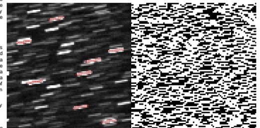
Fig. 6. Left: simulated PASS star field for an exposure of 60 seconds. The size of the field is about  $2 \times 2$  degree. The brightest star is of 4th mag, several have 6-7 mag, and the faintest ones are 14-15mag. The red boxes over the brightest stars show how the aperture mask is being built up, starting with the brightest stars. Right: final aperture mask, where the maximum number of non-overlapping traces have been fitted in.
