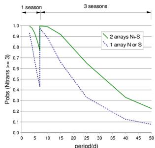
Fig. 5. Probability that transiting planets will be detected by observing at least 3 transits. The green line shows this probability for a configuration of two arrays, based on 650 hours of coverage per year (compare to Fig. 4). The blue line is for a single array, based on 400 hours per year. The left side, for periods up to 7 days, is based on observations from a single season, whereas for periods of 7-50 days, observations spanning 3 years were assumed.
