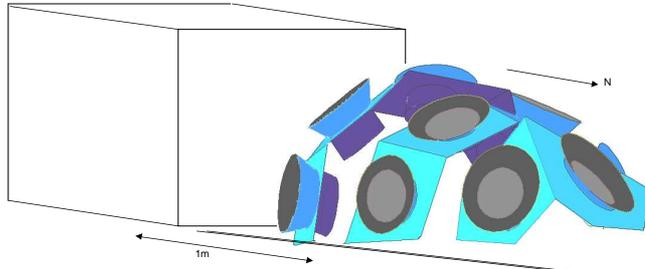
Fig. 1 Schematic view of the PASS experiment, here drawn with 10 cameras. The box in the background is the removable enclosure.
