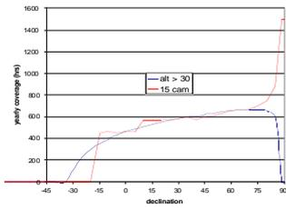
Fig. 3 (on left). Temporal coverage in dependence of declination, assuming a yearly total of 1500 hours of clear observing conditions (200 nights of 7.5 hours) for a site at 28.5°N. Coverage varies much less with right ascension, due to variations in night length and weather conditions throughout a year. The coverage shown here is the average for stars at any right ascension.
