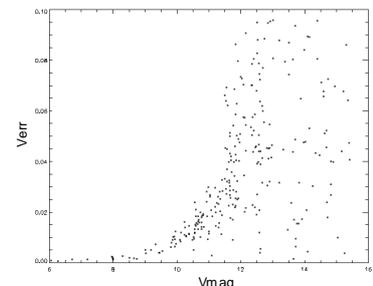
Fig. 7. Photometric error that has been achieved in 10 simulated images with the apertures of Fig. 5. Errors that are  $\leq 0.005$  result from the blending of a bright star within a faint star's aperture. Photometric errors suitable for transit-detection can be expected up to  $V < 11$ .
