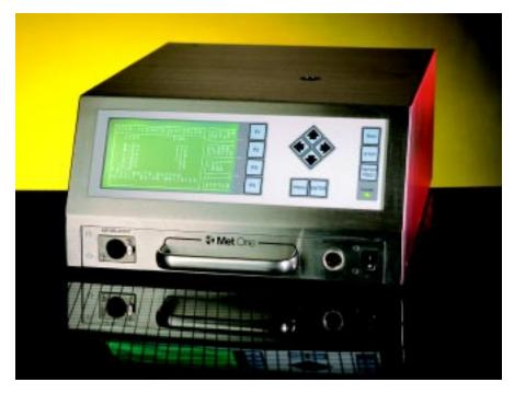
Met One's Model 3313 and Model 3315 deliver a 1.0 cfm (28.3 lpm) sampling rate with either 0.3 micron sensitivity (3313) or 0.5 micron sensitivity (3315). Operating from either AC mains or batteries, the Model 3300 series can provide continuous monitoring of clean areas, storing up to 2000 readings in its memory buffer. The stored data can be reviewed on the front panel, printed, or downloaded to a computer. The built-in printer is standard.
