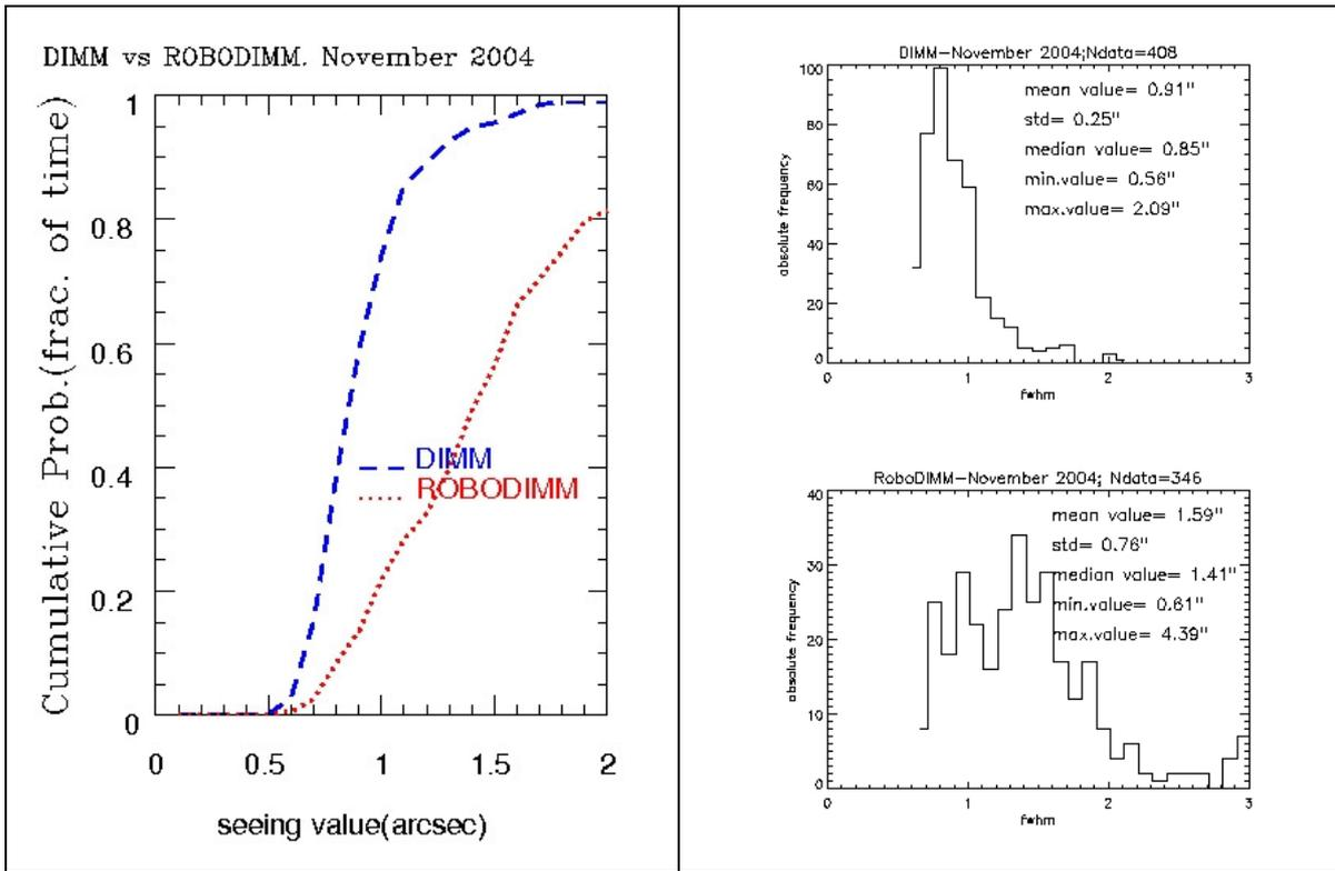
Figure 3a. Cumulative frequency (left) and statistical distribution (right) of the seeing data gathered by the DIMM and RoboDIMM for all possible common nights in November 2004.
