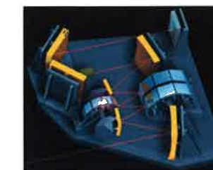
Figure 4: Instruments for space must be strong and compact. Notice the exclusive use of refractive optics and spectral assortment wheels.
