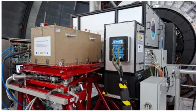
Figure 20. Adaptive optics system installed on the Nasmyth platform of the GTC.
